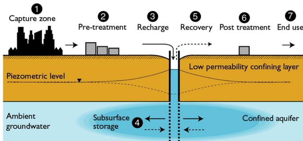
**Figure 3 Seven elements common to all managed aquifer recharge projects (shown for a confined aquifer) (NRMCC-EPHC-NHMRC, 2009a).**
