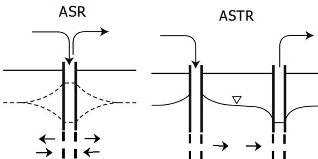
**Figure 2 Schematic illustrating Aquifer storage and recovery (ASR) where a single well is used for injection and recovery and Aquifer storage transfer and recovery (ASTR) where separate wells are used for injection and recovery.**
