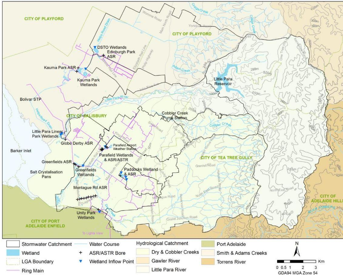
**Figure 1** Salisbury stormwater harvesting catchments and managed aquifer recharge (MAR) schemes showing the location of the Parafield wetlands and MAR (ASR/ASTR) schemes (Page *et al.*, 2013). ASR=Aquifer storage and recovery; ASTR=Aquifer storage transfer and recovery.
