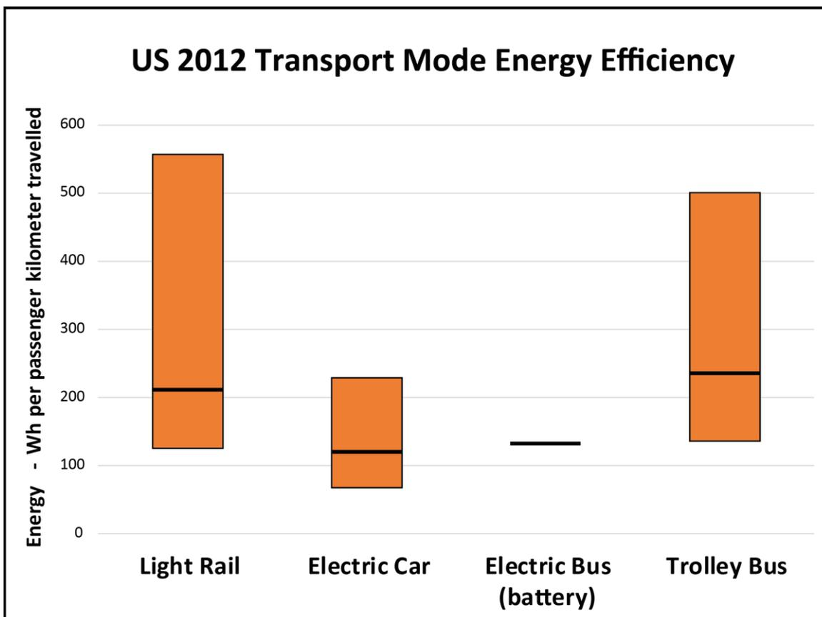
Figure 3 Comparison of four modes of transport based on energy required per passenger kilometre travelled; electric light rail, car, bus and trolley bus. The range in light rail and trolley buses are the range in 2012 US-State averages. The range in electric cars is the range in individual trips. No range was reported for the electric bus trial.
