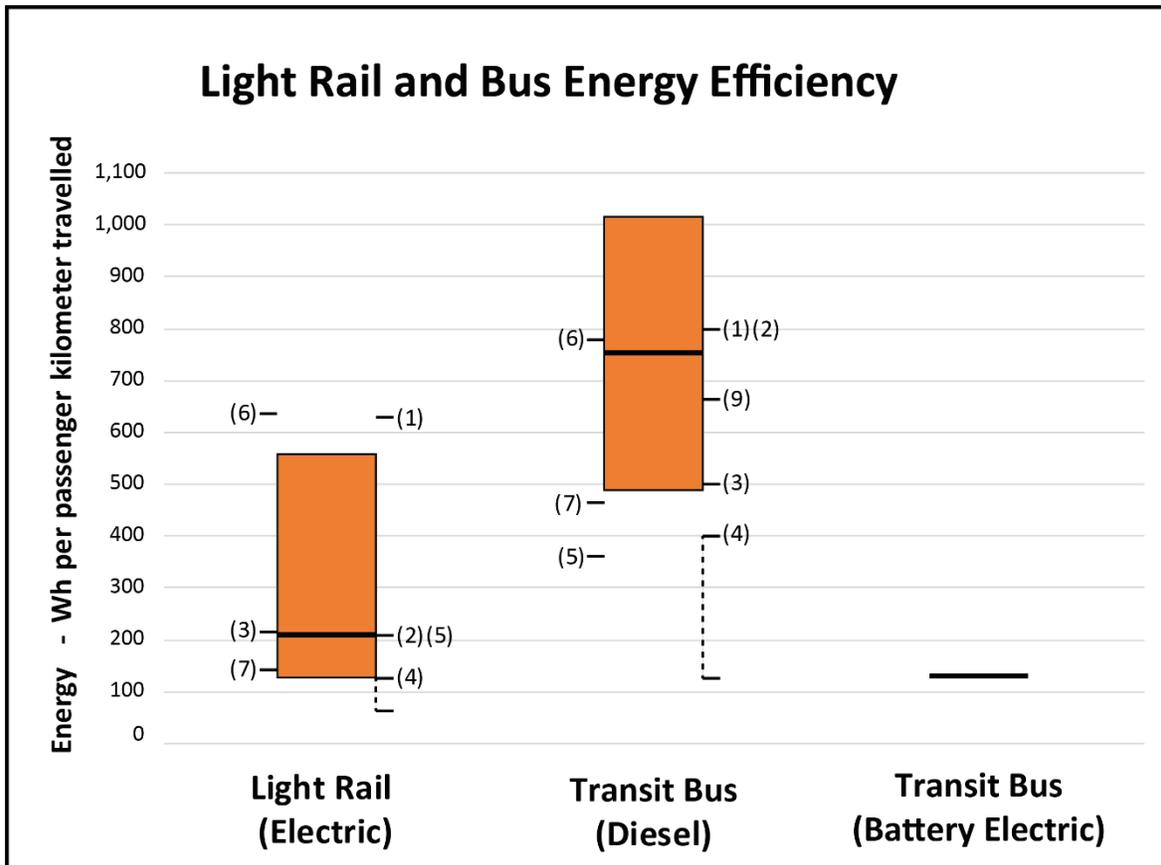
Figure 2 Energy consumption per passenger kilometre for electric light rail and diesel and electric buses. Comparisons based on heating energy consumption. Numbering indicates other authors values: (1) O'Toole (2008); (2) Shapiro et al. (2002); (3) Vincent and Jerram (2006); (4) Potter (2003); (5) Chester (2008); (6) Davis et al. (2014); (7) Kenworthy et al. (1999).
